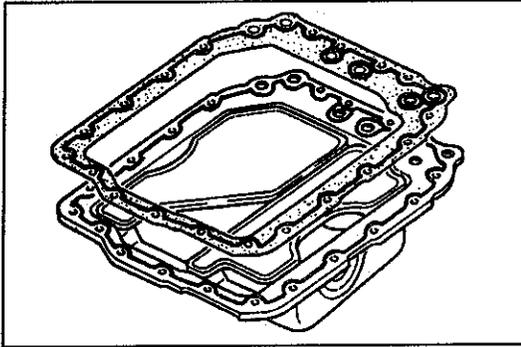
2. Apply silicone sealant to the contact surfaces of the oil pan and the engine side of the new gasket.
