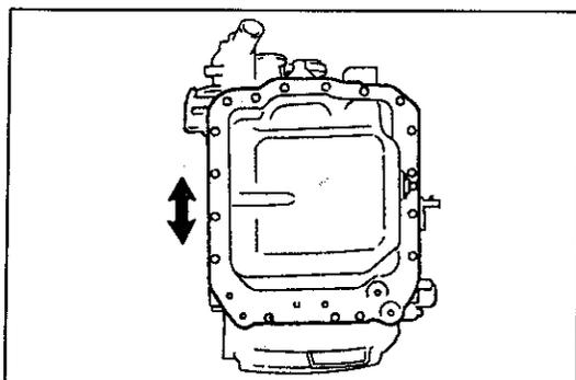
4. Insert a screwdriver only between the points shown in the figure to pry the oil pan loose.
