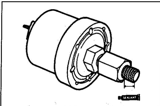
7. Apply sealant to the oil pressure sensor threads. Do not allow sealant in the pressure sensor hole.
