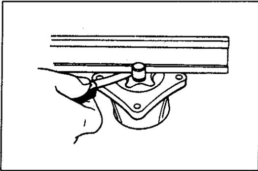
4. Inspect the side clearance of the rotors.
