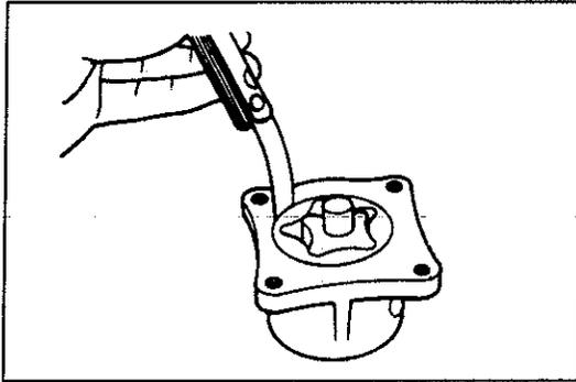
3. Measure the clearance between the outer rotor and the pump body.
