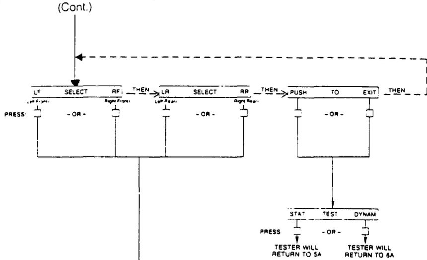
**NOTE: FOR EACH OF THE WHEEL TESTS, IT IS NECESSARY TO RAISE THE WHEEL(S) BEING TESTED OFF THE FLOOR. (WHEN TESTING REAR WHEELS, BOTH WHEELS MUST BE RAISED OFF THE FLOOR.) AN ASSISTANT WILL BE REQUIRED TO SPIN THE WHEELS.**
