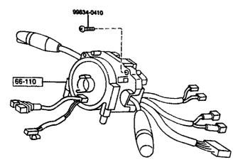
The inner parts of the combination switch with air bag are not serviced separately.
