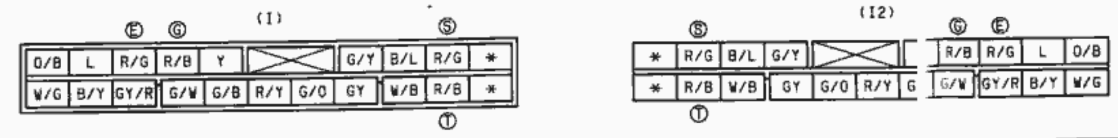
X-19 CONNECTOR BETWEEN DASH (D) & REAR (R)
