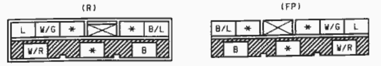
X-24 CONNECTOR BETWEEN REAR (R) & FUEL PUMP (FP)
