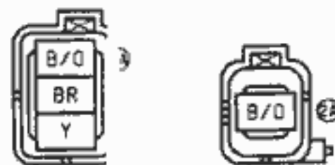
S-08 CONNECTOR BETWEEN DASH(D) & AIR BAG(AB)
