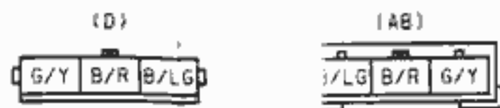
S-08 CONNECTOR BETWEEN DASH(D) & AIR BAG(AB)
