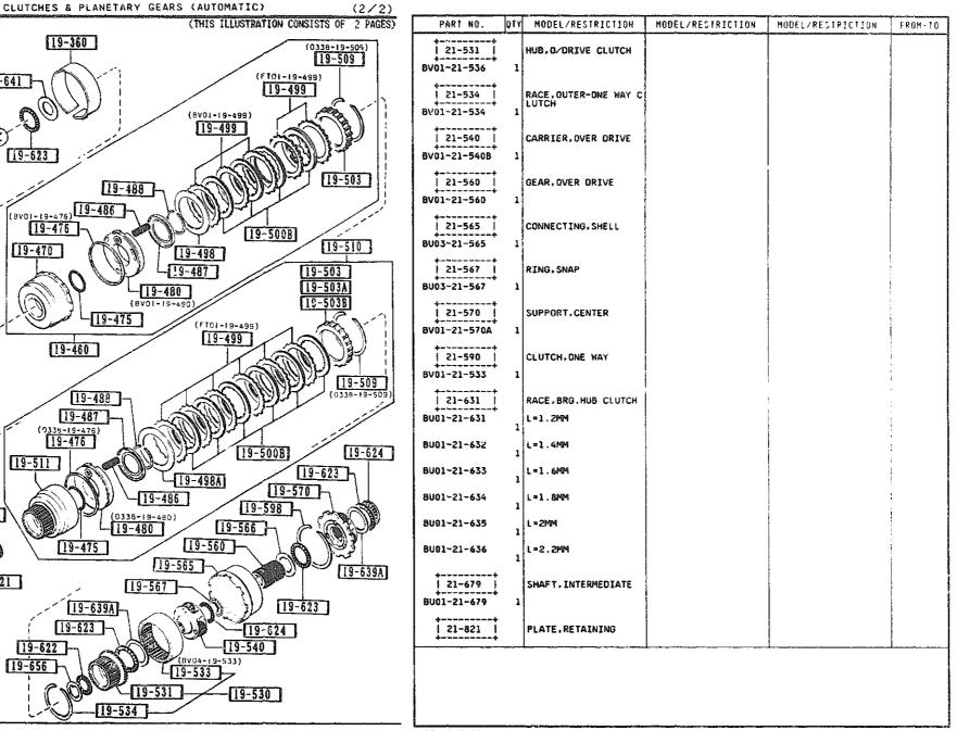
CLUTCHES & PLANETARY GEARS (AUTOMATIC)
