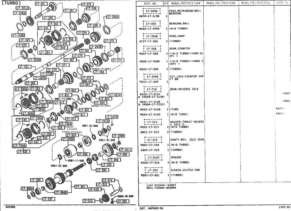
TRANSMISSION GEARS (MANUAL) (THIS ILLUSTRATION CONSISTS OF 2 PAGES) 1710
