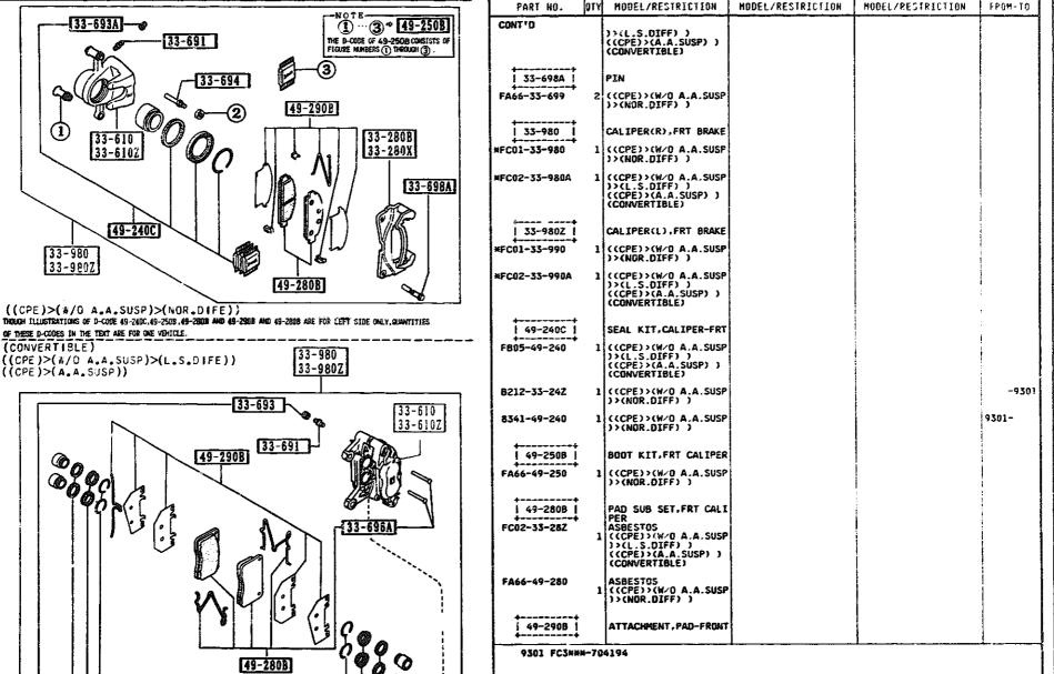
49-240C THOUGH ILLUSTRATIONS OF D-COBE 49-240C.49-2808 MAD 49-2908 ANE FOR LEFT SIDE ONLY, QUANTITIES OF THESE D-CODES IN THE TEXT ARE FOR ONE VEHICLE.
