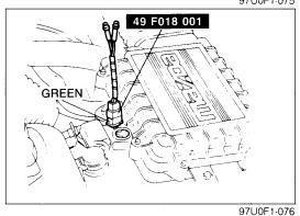
6. Note the operation of the red lamp of the **SST** and the presence or absence of vacuum at that vacuum is felt.
