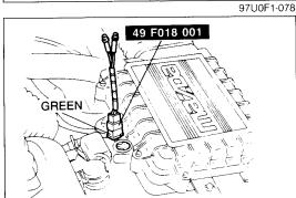
6. Note the operation of the green lamp of the **SST** and the presence or absence of vacuum at that vacuum is felt.
