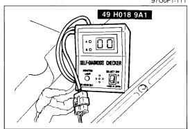
2. Connect the **SST** to the check connector (Green: 6-pin).
