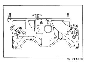
6. Remove the intake manifold.
