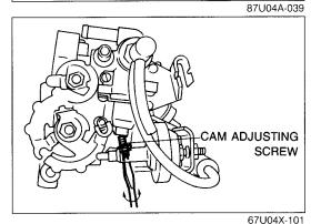
2. If the matching mark and the center of the cam roller do not align, turn the cam adjusting screw until proper alignment is obtained.
