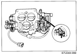
3. If the clearance is not within the specification, bend the tab until the proper clearance is obtained.
