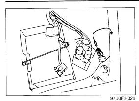
1. Ground the test connector (Green: 1-pin).
