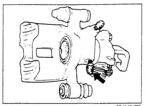
After disassembling the caliper: Bleed air by using the lower bleeder screw. Air bleeding procedure is done in the same manner as the air bleeding of the front brakes.
