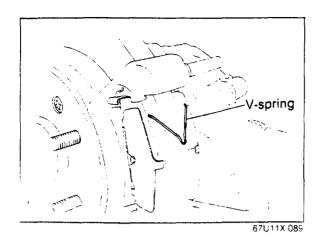
**V-Spring**Install the V-spring to the pads as shown.
