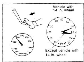
Start the engine. Depress the brake pedal when the vacuum reaches 500 mm-Hg (19.7 in-Hg). If the relationship between the pedal force and fluid pressure is as specified, the unit is functioning.
