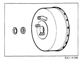
9. Put the dust seal and retainer into the front shell.
