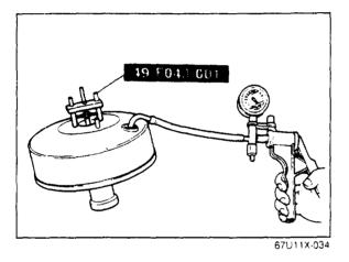
2. Apply **500 mm-Hg (19.7 in-Hg)** vacuum using a vacuum pump.
