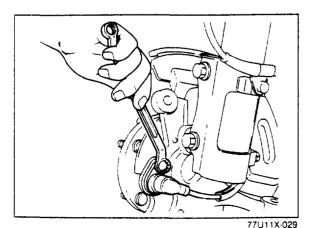
Remove the attaching bolt and remove the speed sensor from the knuckle.
