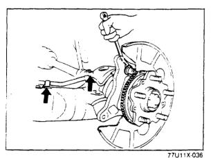
Installation of Speed Sensor
