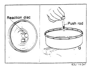
8. Push the reaction disc into the power piston using the push rod.
