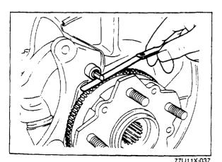
2. Check the clearance between rotor and pick-up of the speed sensor.
