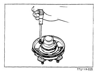
3. Remove the screws and remove the rotor from the wheel hub.
