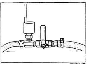
HOW TO USE THE MULTI-PRESSURE TESTER When inspecting the fuel pressure, use the Multipressure tester (49 9200 750A).
