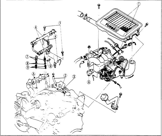
Remove the parts in the sequence shown in the figure.
