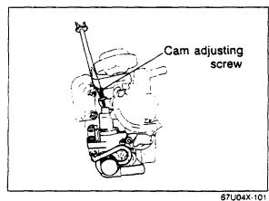
2. If the matching mark and the center of the cam roller do not align, turn the cam adjusting screw until proper alignment is obtained.
